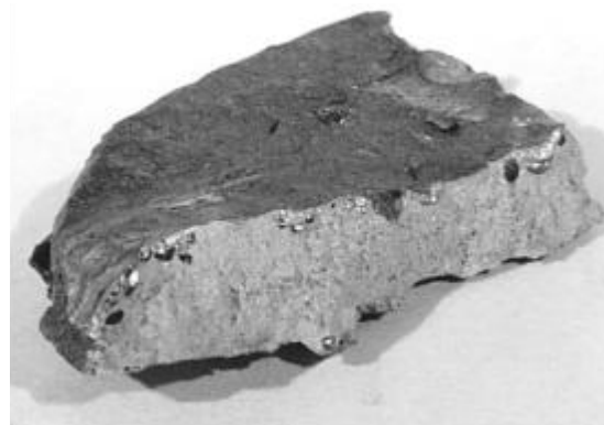
Fig. 2. Copper obtained in case of adding 15 % CaO, 10 % CaF 2 and 100 % reducer
