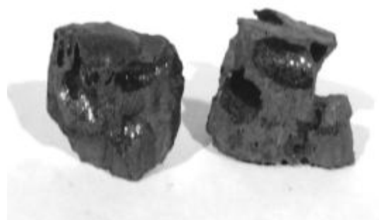
Fig. 3. Slag obtained in case of adding 15 % CaO, 10 % CaF 2 and 100 % reducer.
