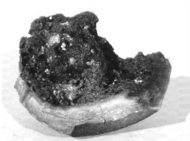
Fig. 1. Viscous, nonhomogeneous slag with copper drops.
