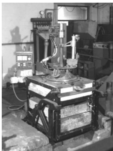
Fig. 4. 50-kg Laboratory Plasma-Induction Furnace "PLASMALAB" [9].
