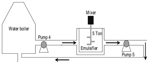
Fig. 2. Schematic diagram of the heating cycle for aqueous-emulsion process.
