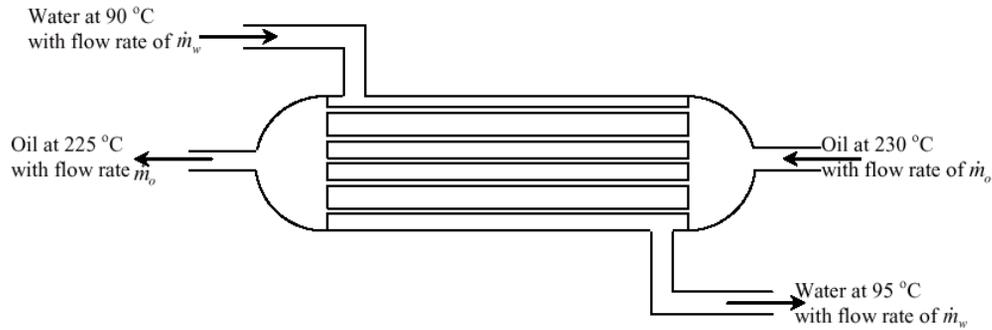
Fig. 5. Schematic diagram of the heat exchanger with its inlet and outlet streams.
