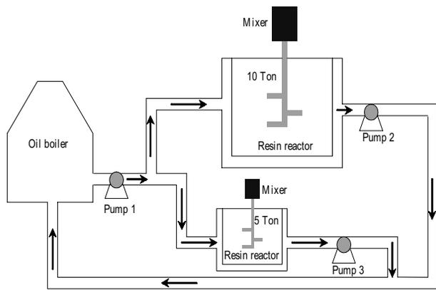
Fig.1. Schematic diagram of the heating cycle for alkyd-resin process.
