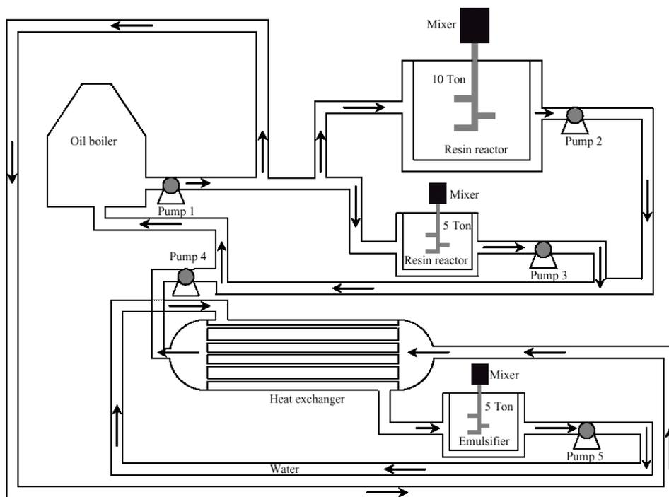
Fig. 3. Schematic diagram of the heat-integrated cycle for alkyd-resin and aqueous-emulsion processes.
