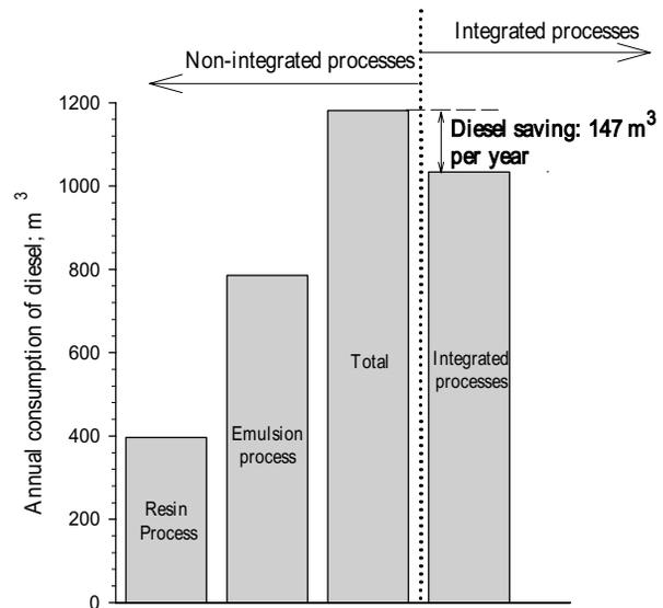
Fig. 4. Comparison between non-integrated and integrated processes of the Jordanian paint company (High Quality Company; Amman). Note that 1 year = 300 operating days.
