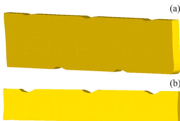
Fig. 5. The profile of the workpiece after rolling in smooth rolls: (a) the first scheme; (b) the second scheme.
