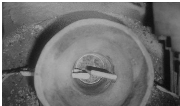
Fig. 4. Location of the thermocouples in the volume of the ingot.
