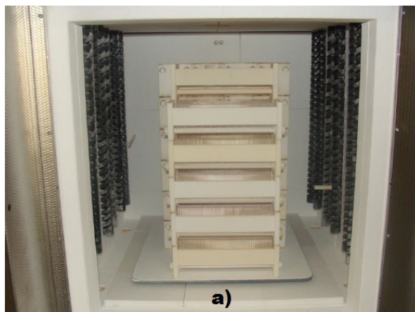
Fig. 7. Common view of the arrangement in sintering: a) the first platinum layer 34 (horizontal) ceramic holders; b) the second platinum layer 22 (vertical) ceramic holders.
