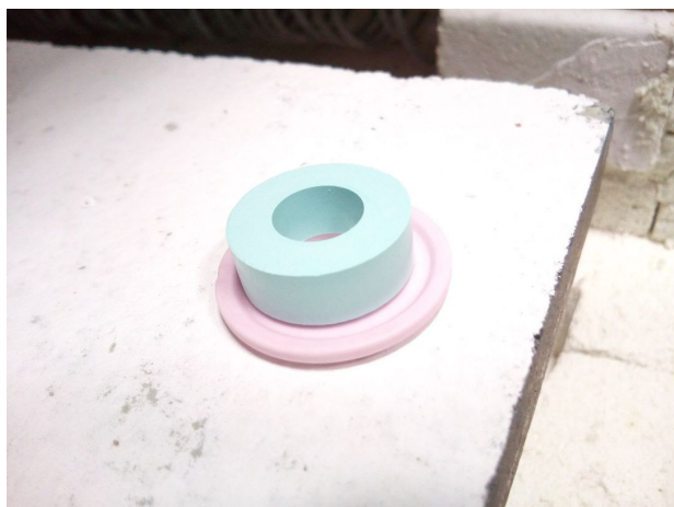
Fig. 6. Common view of shrink ring on a ceramic washer.
