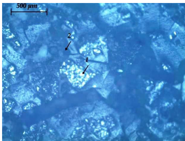
Fig. 13. Microstructure of the obtained briquettes for Mixture 1 (1:1 ratio); 1- \text{Fe}_3\text{O}_4 , \text{Fe}_2\text{O}_3 , \text{FeO} ; 2 - silicate connection (Olivine).
