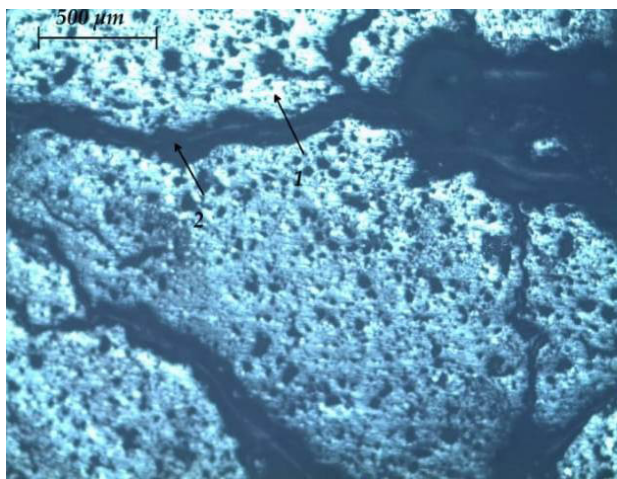
Fig. 14. Microstructure of the obtained briquettes for Mixture 2 (1:10 ratio); 1- \text{Fe}_3\text{O}_4 , \text{Fe}_2\text{O}_3 , \text{FeO} ; 2- silicate connection (Olivine).
