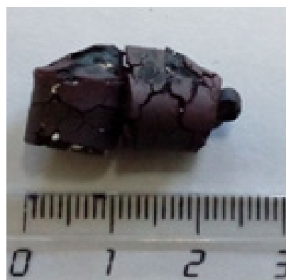
Fig. 9. Briquettes heated at T = 1150^\circ\text{C} in 1:1 ratio.
