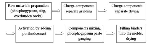
Fig. 2. Technological scheme for obtaining an unburned mineral binder.
