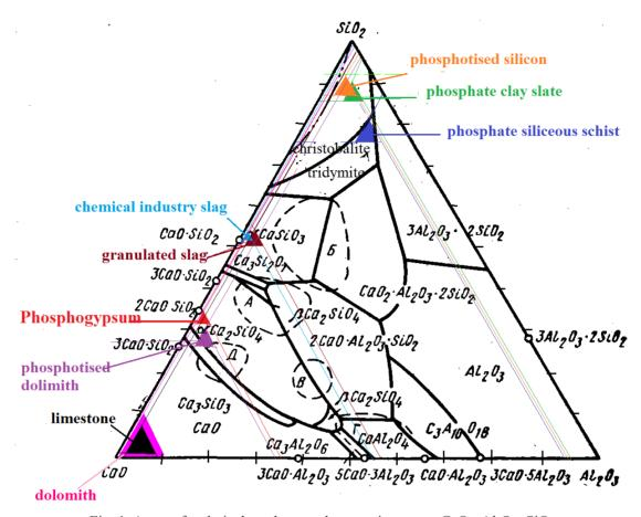
Fig. 1. Areas of technical products and wastes in system CaO - Al<sub>2</sub>O<sub>3</sub> -SiO<sub>2</sub>.
