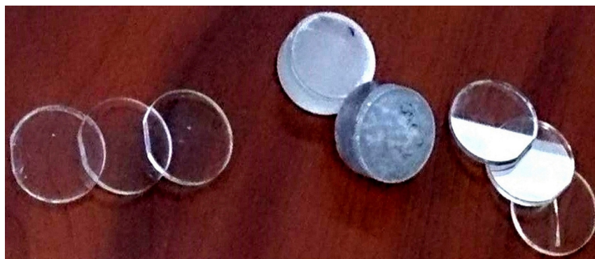
Fig. 1. Crystals and finished lasing windows ( 1'' \times 2.9 \text{ mm} \pm 0.1 ): the brighter boule upper and the windows on left - 1.8 % ( \text{YbF}_3 ), 2.5 % ( \text{NaF} ): \text{CaF}_2 ; the darker boule down and the windows on right - 1.8 % ( \text{YbF}_3 ), 2.5 % ( \text{NaF} ): \text{Ca}_{0.67}\text{Sr}_{0.33}\text{F}_2 .
