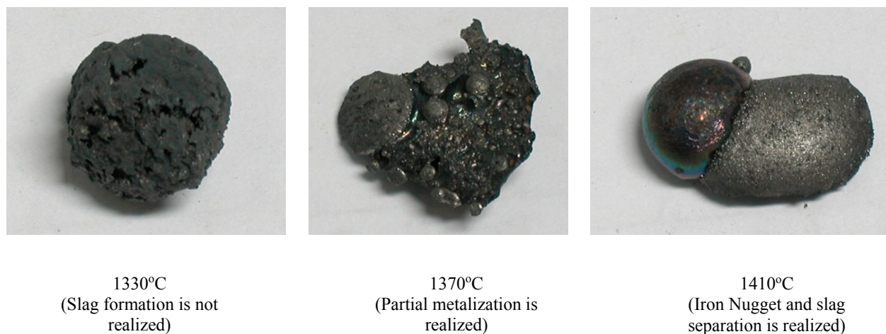
Fig. 2. Macro images of products obtained from carbon composite pellets treated for 8 minutes in different furnace temperatures.
