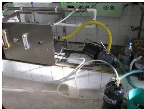
Fig. 1. Principle scheme of the cross-flow UF system used.
