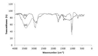
Fig. 7. FTIR spectra of (a) palm olein oil and (b) palm olein oil biodiesel.
