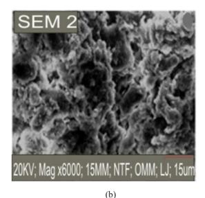
Fig. 2. SEM images of (a) raw and (b) calcined anthill.
