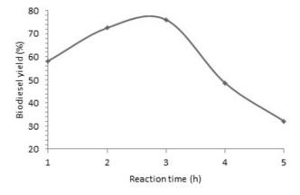
Fig. 5. Biodiesel yields at different reaction time at fixed reaction temperature =  $70^{\circ}$ C, catalyst dose = 2.0 wt. % and methanol/oil molar ratio of 6:1.
