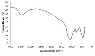
Fig. 3. FTIR spectrum of calcined anthill.
