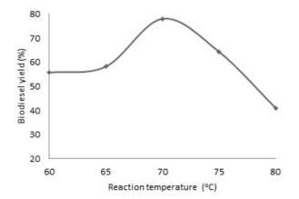
Fig. 4. Biodiesel yields at different reaction temperatures at fixed reaction time = 3 h, catalyst dose = 2.0 wt. % and methanol/oil molar ratio of 6:1.
