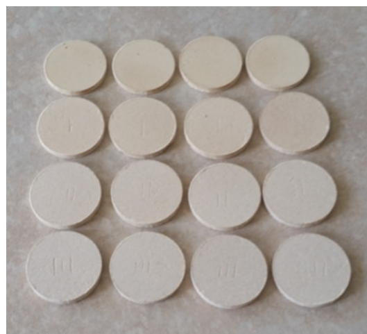
Fig. 1. Ceramic membranes sintered at 1100°C.
