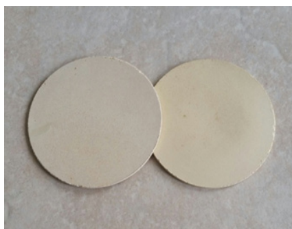
Fig. 3. Ceramic membrane support, fired at 900°C, and ceramic membrane fired at 800°C.
