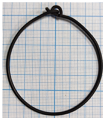
Fig. 1. Ring-shaped force element made from Ti - 50.5 at. % Ni alloy.
