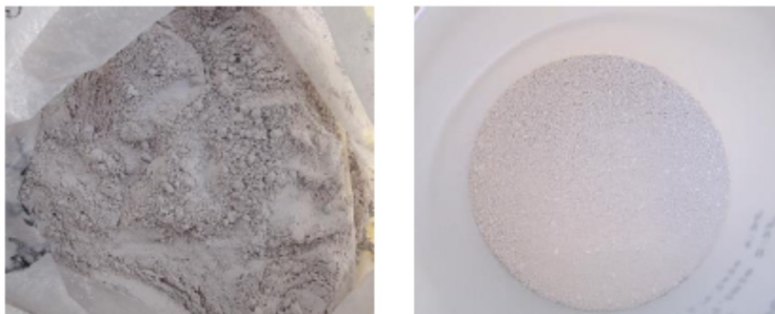
Fig. 3. Comparison of brightness; left: raw barite with particle size 40 \mu\text{m} , right: the same barite after calcination.
